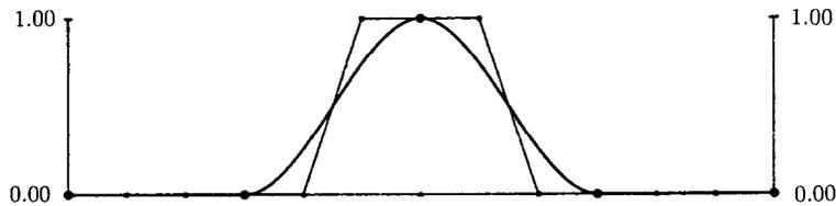
Fig. 19. Basis function: uniform  $\gamma = 0$ .
