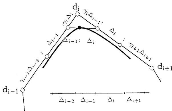
Fig. 1. A free-form  $\gamma$ -spline.
