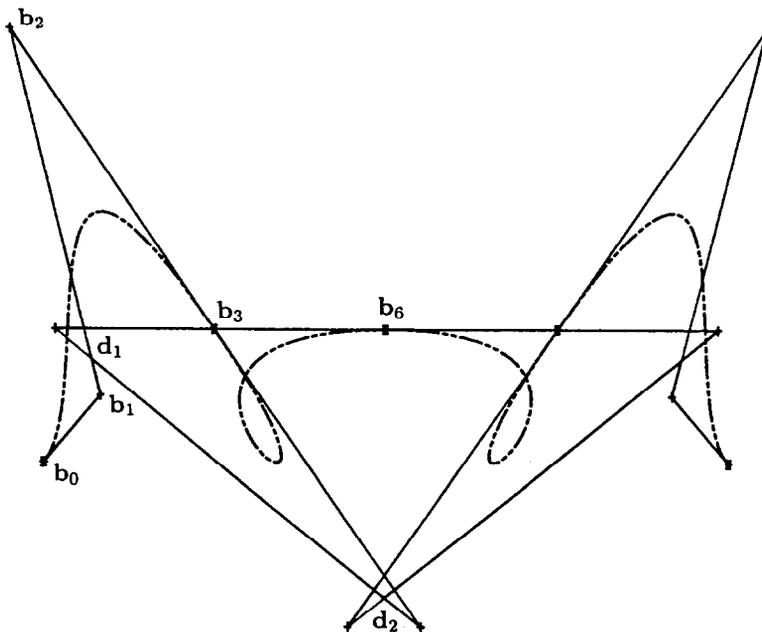
Fig. 13. Interpolating  $\gamma$ -spline with  $\gamma_i = -0.9$  for all  $i$ ; this is very close to an eigenvalue singularity.
