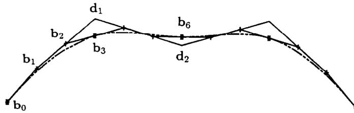
Fig. 10. The  $C^2$  interpolating  $\gamma$ -spline where  $\gamma_i = 1$  for all  $i$ .
