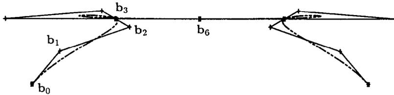
Fig. 12. Interpolating  $\nu$ -spline with  $\nu_i = (0, -24, 0)$ ; this curve cannot be represented as a  $\gamma$ -spline.
