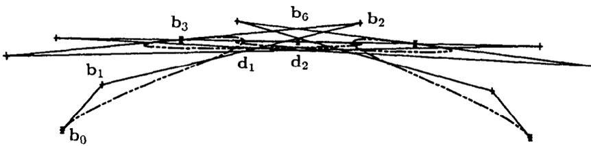
Fig. 15. Interpolating  $\gamma$ -spline with  $\gamma_i = -0.45$  for all  $i$ .
