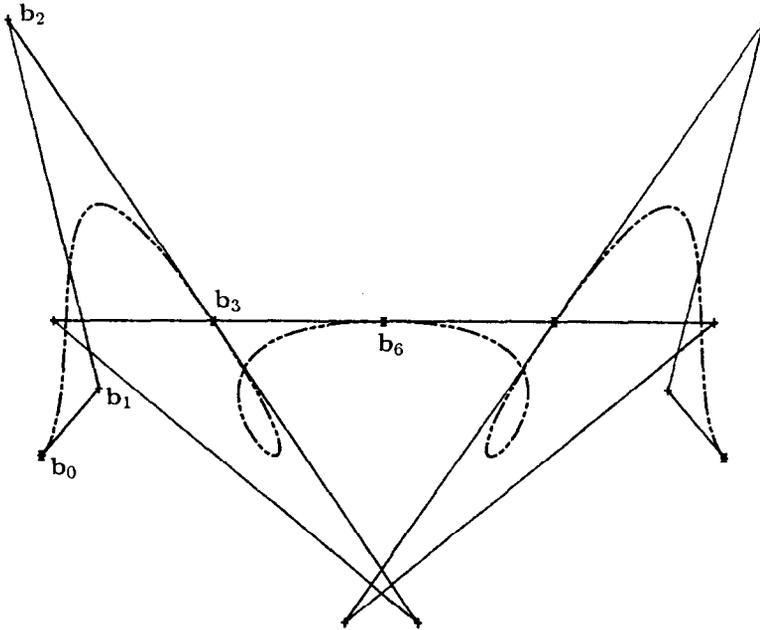
Fig. 14. Interpolating  $\nu$ -spline with  $\nu_i = -33.7$  for all  $i$ ; this is the same curve as in previous figure.
