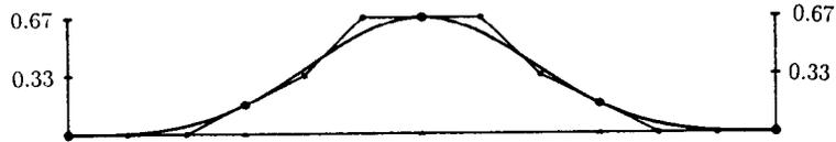
Fig. 17. Basis function: uniform  $\gamma = 1$ .
