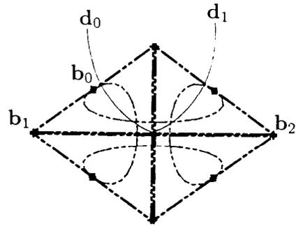
Fig. 5. Interpolating to four points with uniform  $\gamma = -0.45$  and uniform knot spacing.
