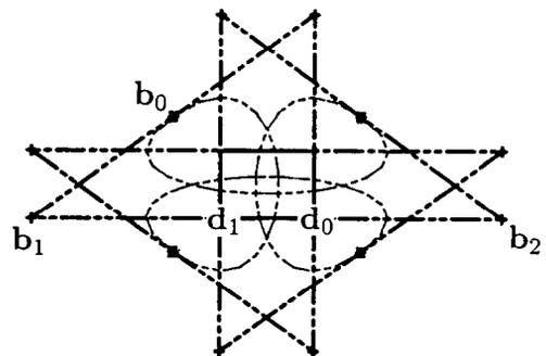
Fig. 7. Interpolating to four points with uniform  $\gamma = -0.6$  and uniform knot spacing.
