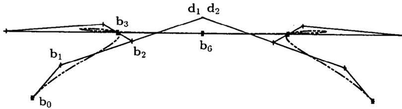
Fig. 11. Interpolating  $\gamma$ -spline with  $\gamma_i = (1, -1.99, 1)$ ; this curve is very close to a  $\delta = 0$  singularity.
