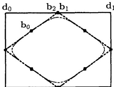
Fig. 9. Interpolating to four points with uniform  $\gamma = -40$  and uniform knot spacing.
