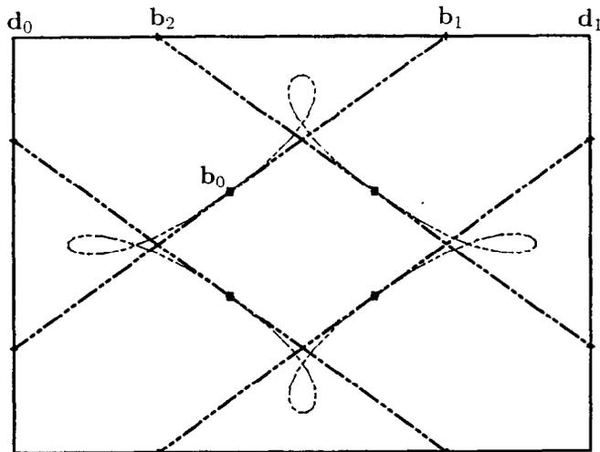
Fig. 8. Interpolating to four points with uniform  $\gamma = -1.5$  and uniform knot spacing.
