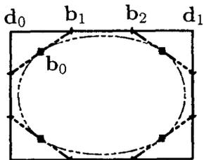
Fig. 2. Interpolating to four points with uniform  $\gamma = 1$  and uniform knot spacing.
